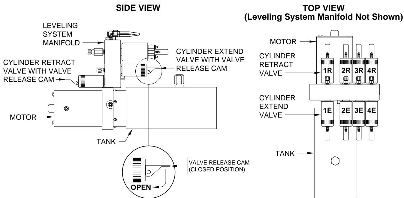
**IMPORTANT: Open both the Cylinder Extend and Cylinder Retract valves for a room to release pressure before replacing one or both valves for that room. Turn the Valve Release Nuts NO MORE THAN 4 1/2 full turns counter clock wise to open the valves. Remember to close the valve(s) after the repair is complete. Tighten the Valve Release Nuts snug only. DO NOT over tighten.**
