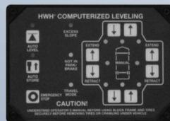
← 725 Series computer-controlled, fully automatic system, the simplest and most effective way to level your coach. Touch Panel is usually floor mounted. (Optional dash bezel available)
