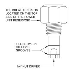
IMPORTANT: PRIOR TO REMOVING THE BREATHER CAP, EITHER TO CHECK THE OIL LEVEL OR TO USE 1/4" NUT DRIVER, CLEAN ANY DEBRIS FROM THE TOP OF THE RESERVOIR. BEFORE RETURNING THE BREATHER CAP TO THE RESERVOIR, REMOVE ANY PAINT CHIPS OR OTHER DEBRIS FROM THE DIPSTICK INCLUDING DEBRIS INSIDE THE 1/4" NUT DRIVER.
